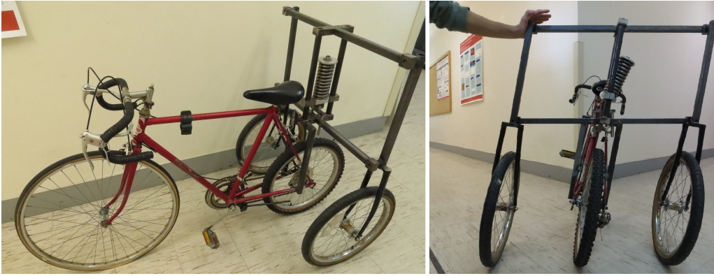
Figure 1. A ‘bricycle’: a vehicle which can transition between bicycle and a tricycle. It is a bicycle with two extra ‘training’ wheels at the back on a spring-loaded parallelogram mechanism. The spring resists bicycle lean, more or less depending on its adjustment. When the spring is removed the training wheels are mechanically invisible, effectively reducing the bricycle to a bicycle. When the spring is locked the bricycle is effectively a tricycle. The neutral point in-between, when the spring is such that the bricycle is in equilibrium at all small angles of lean, is the main topic of study here.
