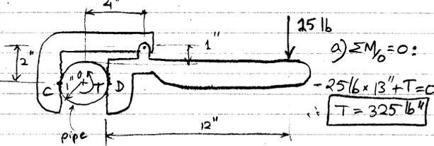
$$\begin{aligned} \sum M_D = 0: \\ -25 \times 13 + T = 0 \\ \Rightarrow T = 325 \text{ lb} \end{aligned}$$
