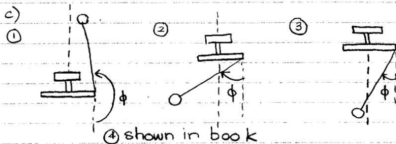
8.44 A rod is attached to a shaft which spins @ constant rate  $\omega$  about the z-axis. There is a ball and socket joint @ A and B is held by 2 strings connected to a crossbar.
