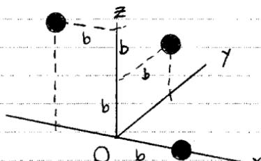
$$[I^\circ] = [I^{CM}] + m \begin{bmatrix} y_{CM/0}^2 + z_{CM/0}^2 & -x_{CM/0} y_{CM/0} & -x_{CM/0} z_{CM/0} \\ -x_{CM/0} y_{CM/0} & x_{CM/0}^2 + z_{CM/0}^2 & -y_{CM/0} z_{CM/0} \\ -x_{CM/0} z_{CM/0} & -y_{CM/0} z_{CM/0} & x_{CM/0}^2 + y_{CM/0}^2 \end{bmatrix}$$
