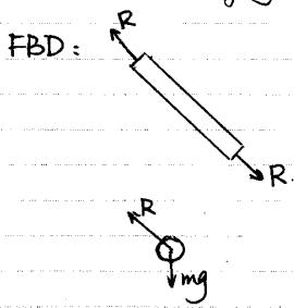
If one includes the ball, the system does not form a two force member (like part a).
