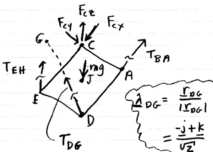
b) Consider the axis DE. The only forces w/ non zero moment are  $mg$  at H and  $F_{Cz}$  at C. So
