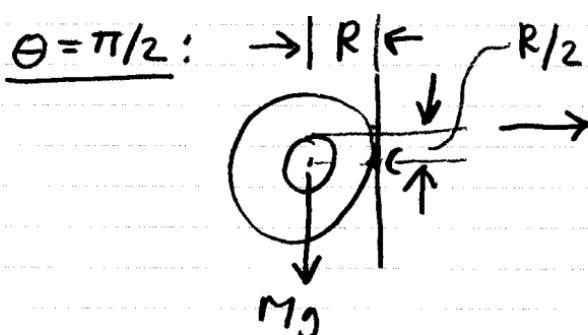
tension has half the lever arm about pt. C  $\Rightarrow T = 2Mg \Rightarrow m = 2M$ .
